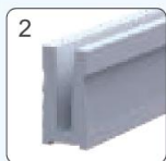
U groove (YM18-04) Material: 6063-T6 Glass Thickness: 13.5/17.5mm Length :L≤6000mm
